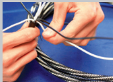
Hands-on at the customer’s request: Taken for granted, in-akustik tailor individual lengths. Not to be taken for granted: a single to bi-wiring separation of conducting paths. A splitter of massive aluminium is inserted between the supply and return conductors in order to keep inductivity low.
