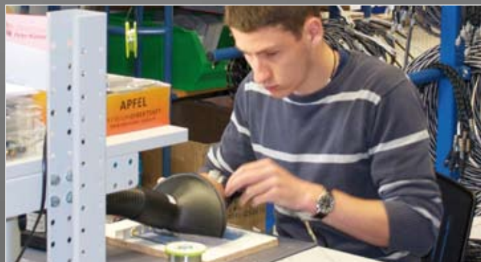
The complex cable structure calls for steady hands while attaching plugs. An extractor draws off solder fumes created in the process.
